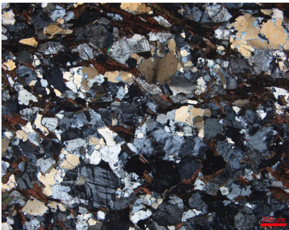
Pmg – 4: Photomicrograph showing association and parallel alignment of microcline, quartz, plagioclase and biotite in granite gneiss as seen under crossed nicols.
